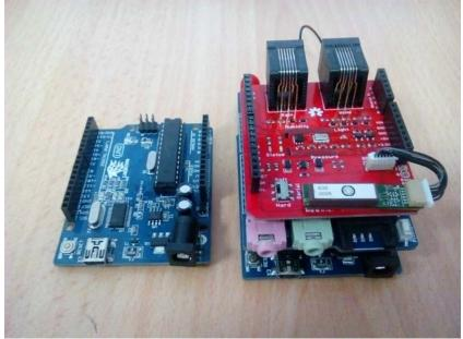
Figure 4: Arduino alone (Left), built with SMS and red weather shields (right)
